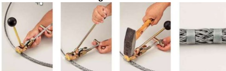
Figure 70 Banding Kellum's Apply Bands at 1" to 2" from the end of the Mesh
